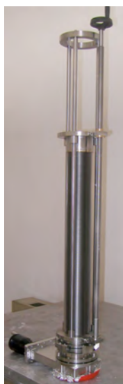
Figure 4: external load lock insert and valve. Figure 5: top cover with the load-lock flange.
