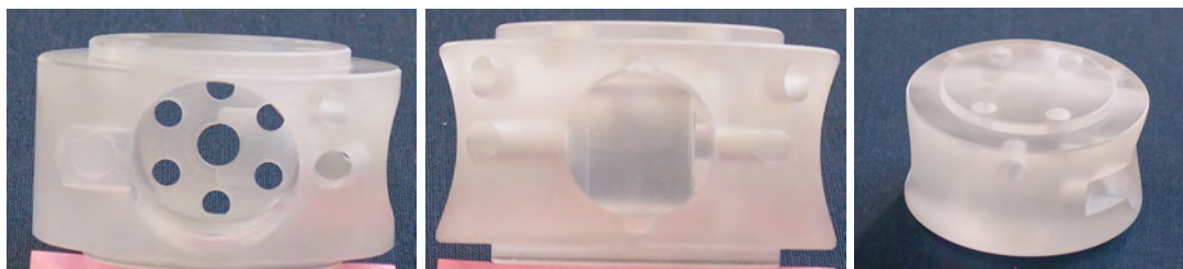
Figure 10: Lateral views of the sapphire sample-holder showing the DAC break (left) and the slider break (central). Top view on the right.
