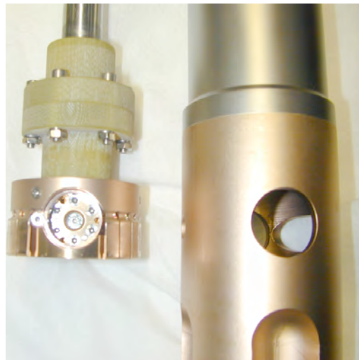
Figure 8: Photographs of the internal sample-holder with the DAC (left), the spring crown for the cold contact (left) and the external fixed part (right).
