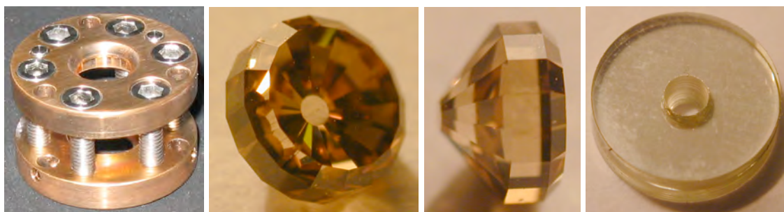
Figure 14: The Cu–Be disks of the DAC with its Ti screws (left), the two diamonds (centre), a moissanite (SiC- \delta ) cylinder with its 400 \mu\text{m} conic hole (right).
